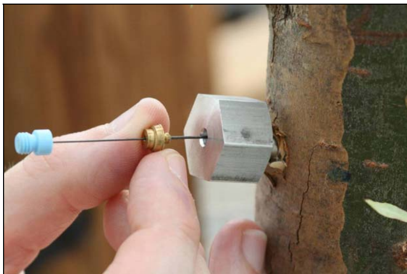
Figure B.3: SPME in-planta application photo from field application of SPME analysis
