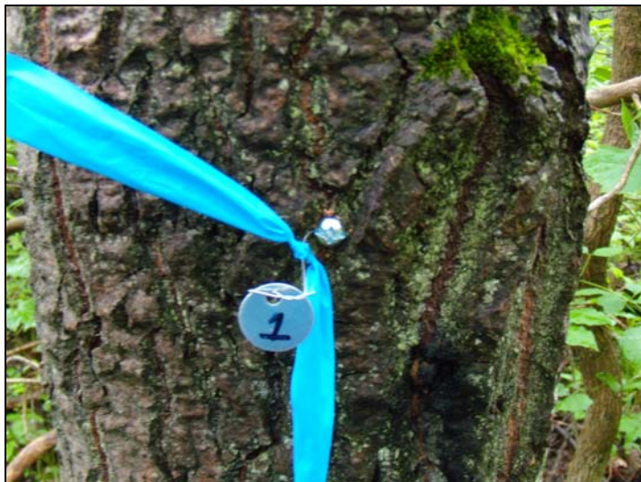
Figure B.5: Once SPS is placed inside open core, a screw used to seal the hole from the outside environment.
