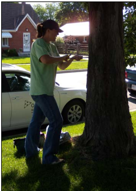
Figure B.1: Core removal from tree on site in Toronto, Canada
